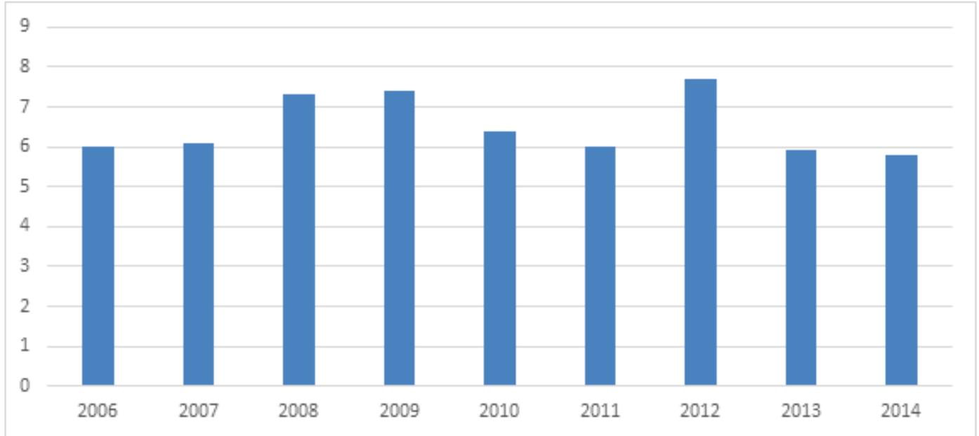
**Figure 2: Average power density (in kW) per rack - Emerson DCUG data from 2006 to 2014**
