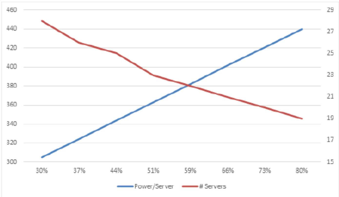
Figure 5: Power per server and Servers per rack vs. CPU usage – 30A 3-phase 208V circuit.
