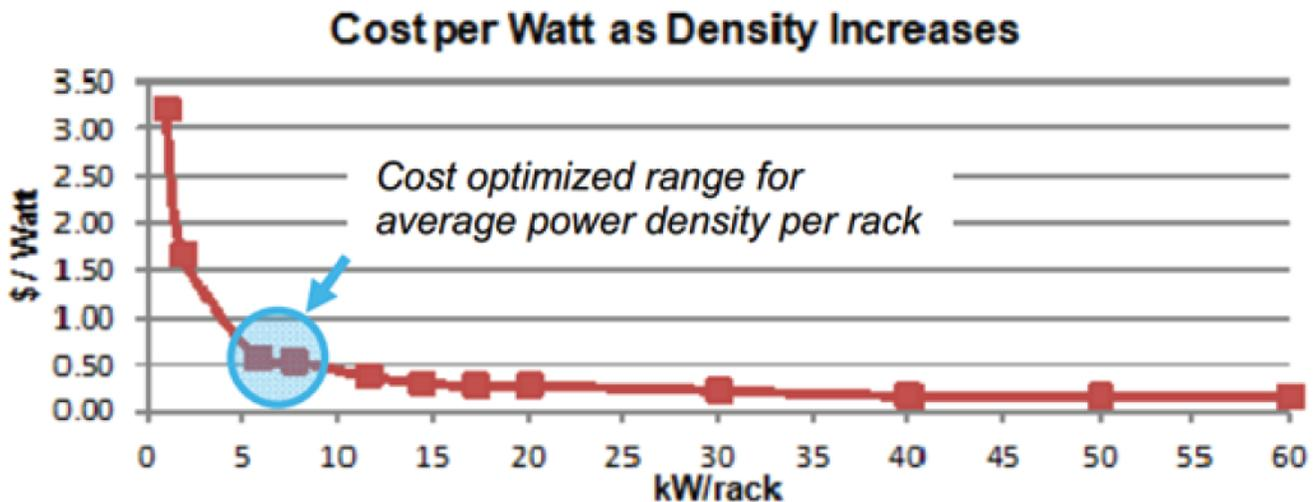
Figure 3: Cost per watt vs power density – Schneider Electric (2014)
